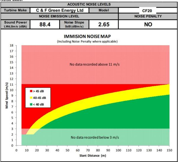
Immission Sound Pressure Levels at 8 m/s hub height wind speed:
